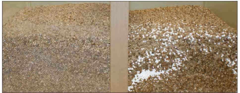
On the left, MAP blended with Boron DDP Micronutrient. Each prill of MAP is coated evenly. On the right, granular Boron settles unevenly through the blend as the blend is handled and transported.
